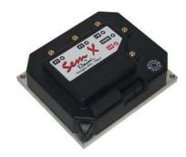
The SEM-X controller is suitable for pallet trucks, floor washing machines and small capacity trucks, equipped with D.C. Separately Excited Motors up to 700W. General features: MOSFET technology, microprocessor logic, faults memory, digital programming via console, regenerative braking.
