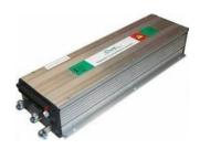
This controller has been developed for reach trucks, medium-sized lift-trucks and tractors, equipped with D.C. Separately Excited Motors within a power range from 6 to 12 kW. General features: MOSFET technology, microprocessor logic, faults memory, digital programming via console, regenerative braking
