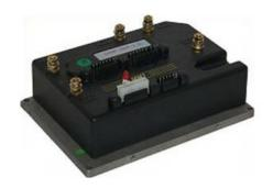
The SEM1 controller has been developed for road traction and for trucks. It is suitable for electrical vehicles, equipped with D.C. Separately Excited Motor, from 1 kW to 3.5 kW. General features: MOSFET technology, microprocessor logic, faults memory, digital programming via console, regenerative braking.
