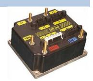
The SEMO controller has been developed for road traction and for trucks. It is suitable for electrical vehicles, equipped with D.C. Separately Excited Motor, from 0.5 kW to 2 kW. General features: MOSFET technology, microprocessor logic, faults memory, digital programming via console, and regenerative braking.
