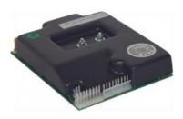
This family of choppers have been designed for control of permanent magnet motors with power from 200 to 800W. This product is suitable for cleaning machines, pallet trucks, golf cars, and small electric vehicles. General features: MOSFET technology, microprocessor logic, faults memory, digital programming via console, regenerative braking.
