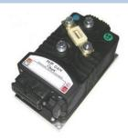
The ZAPI HP CAN is suitable for operations in medium and large capacity vehicles, such as counter balance, order picker, reach and three wheel trucks. It is capable of controlling DC series wound motors from 2kW to 20kW power ranges.
