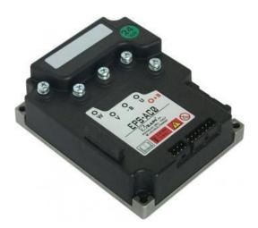
This is a compact and cost effective steer by wire controller for 24/48V trucks fitted with AC steering motors up to 500W. It is suitable for handlebar and tiller trucks. Microprocessor technology, combined with the CAN Bus communication system, provides an effortless steering command facility, with several advanced features:
