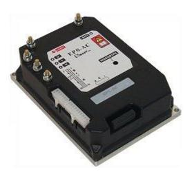
Steer by wire controller for AC steering motors (EPS-AC). ZAPI started the development of DC Electronic Power Steering systems for lift truck applications in 1992. The EPS-AC system reflects ZAPI's experience in the initial DC products together with state of the art asynchronous technology. The EPS-AC is suitable for asynchronous steering motors between 200W and 1kW.
