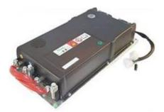
This controller is suitable for twin motors electrical vehicles (3 and 4 wheel trucks), fitted with two separately excited traction motors, with power from 1.5 up to 15 kW. General features: MOSFET technology, microprocessor logic, faults memory, digital programming via console, regenerative braking.
