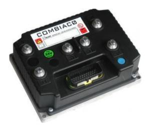
The CombiAC-0 controller is suitable for pedestrian, small stacker trucks, and order pickers fitted with encoderless asynchronous motors up to 2,5 kW, and DC series pump motor up to 5 kW.
