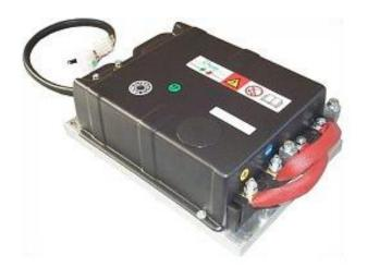
The following functions are fitted in the same box (package): traction control for one separately excited D.C. motor; lifting control for D.C. series excited or compound motor. Power range: 3÷13kW for the traction motor, up to 15kW for the pump motor. General features: MOSFET technology, microprocessor logic, faults memory, digital programming via console, regenerative braking.
